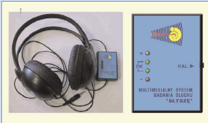
Fig. 4. Headphones and electronic calibrator used by listeners to set the gain of the computer sound card used for an Internet-based hearing assessment.
